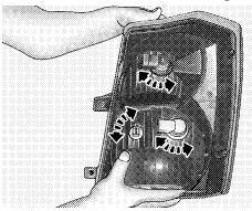
Removing Socket And Bulb
